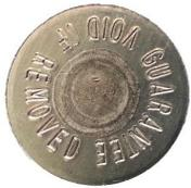
**A heat tab has been installed on each block within a freeze plug. A melted tab indicates the engine has reached a temperature hot enough to do internal damage, and the warranty becomes void. If tab is melted, it is almost always non-warrantable failure.**
